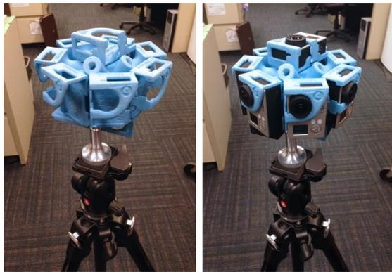
Physical setup consists of mounting the rig on the tripod and inserting the cameras. It requires care, but is straightforward. Of course, each camera needs a charged battery and properly formatted, empty memory. Small details, like lens caps that fit on the cameras when mounted in the rig, make a difference.
